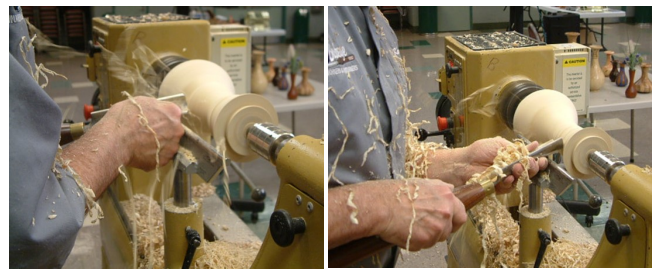
The vessel reversed in the chuck and shaping the outside
