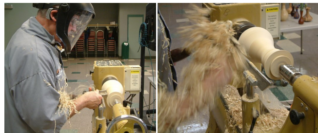
The vessel reversed in the chuck and shaping the outside
