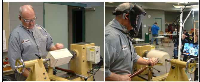
Chucking up a blank and making it round
