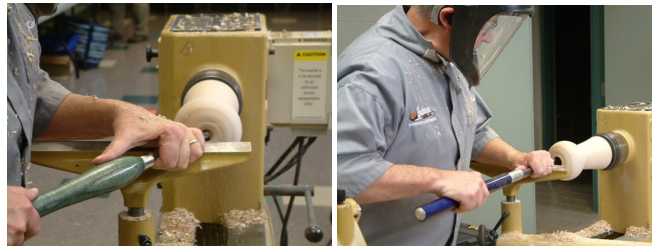
Hollowing the bottom with the lathe in reverse (left) and going forward (right)
