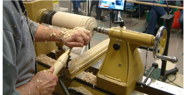
Starting to shape the bottom foot
