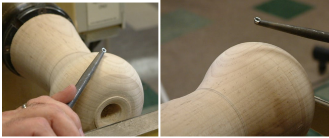
Kevin used a Hunter tool to hollow out the bottom of the vessel
